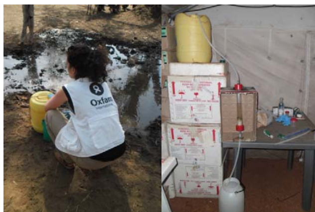
Sampling and concentrating by glass-wool filters
