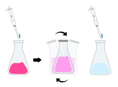
\* **Note:** The reading as 1 mL of the acid solution is equivalent to 1% available lime expressed as CaO.
