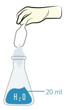
**Step 3.** Cover the flask. Swirl and heat to boiling for 2 mins. Remove from heat
